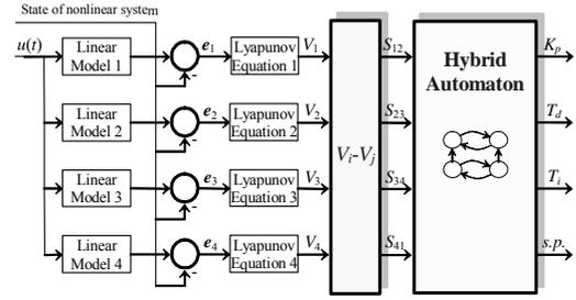
Fig. 5. General scheme for the supervisor
