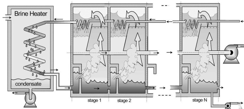
Fig. 1 Schematic representation of a MSF desalination plant
