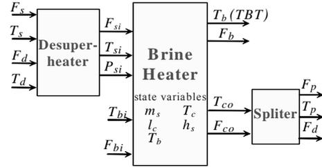
Fig. 3 Variables of the brine heater subsystem
