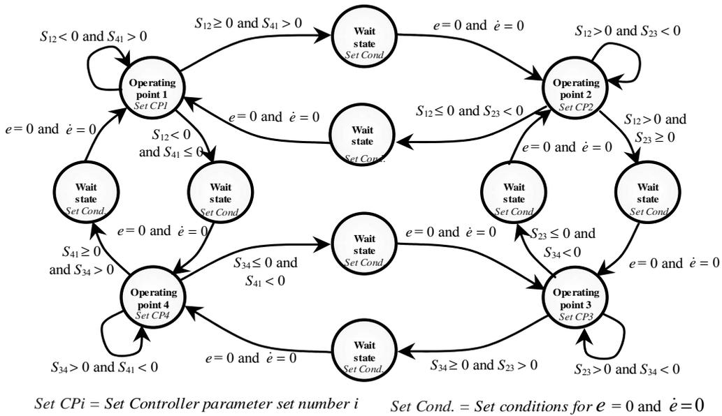
Fig. 7. Stateflow chart for the hybrid automaton
