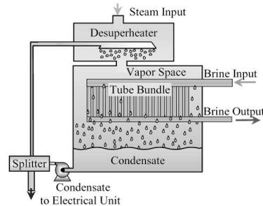
Fig. 2 Schematic representation of the brine heater
